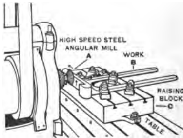
FIG. 25. — MILLING DOVETAIL. PLAIN MILLING MACHINE.
